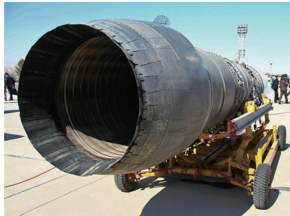
图1 Air Logistics 4000系列发动机安装车 Fig.1 Air Logistics 4000 series engine trailer
