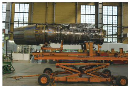
图6 苏-27系列飞机发动机安装车 Fig.6 Engine trailer of Su-27 series fighter
