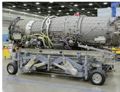
图4 F-35的发动机安装车 Fig.4 Engine trailer of F-35 fighter
