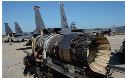
图3 F-15的发动机安装车 Fig.3 Engine trailer of F-15 fighter
